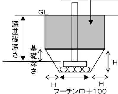
**布基礎埋戻量** = [布基礎根切量] - [布基礎残土処分]
